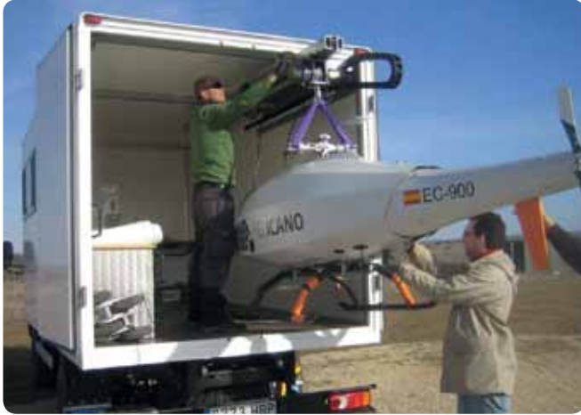
Example of a transport solution for unmanned helicopters.
